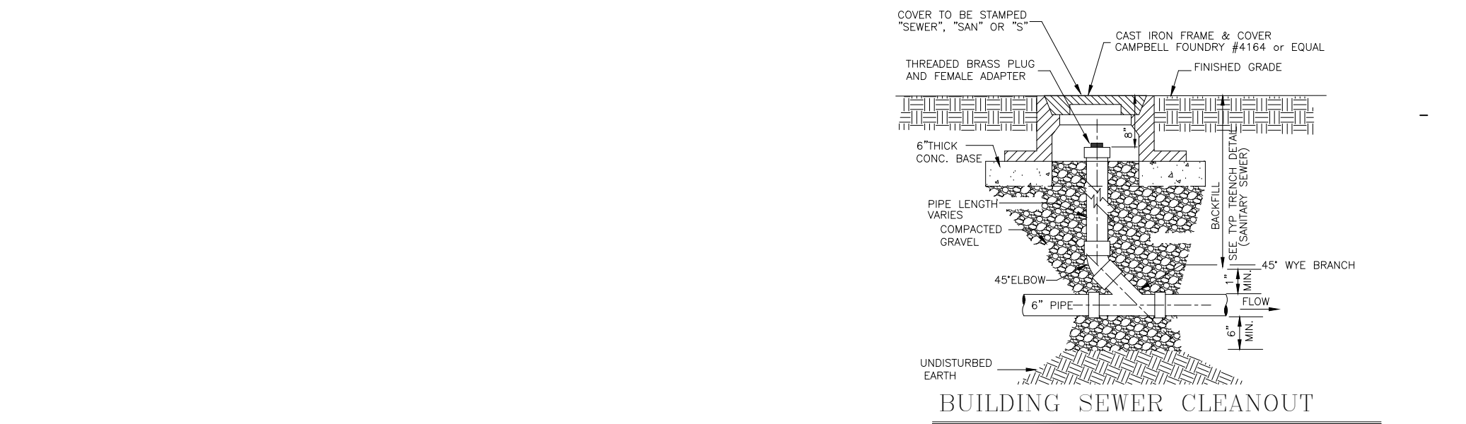
BUILDING SEWER CLEANOUT N.T.S.
