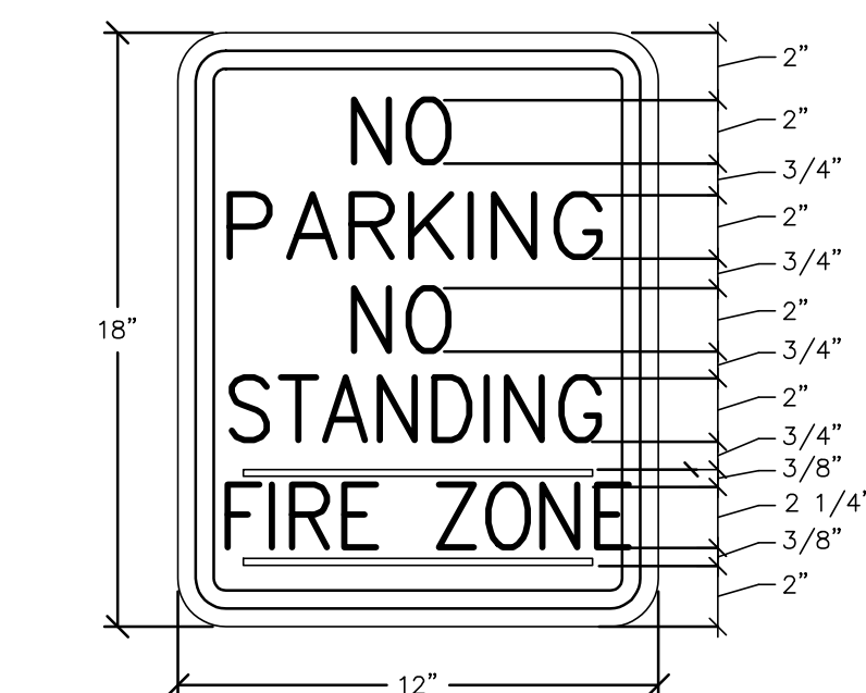
TYPICAL NO PARKING / NO STANDING / FIRE ZONE SIGN DETAIL N.T.S.
